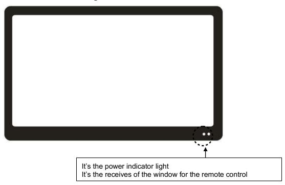
Notice: The power indicator is red for standby mode, and the green is the power supply.
